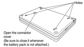
5 Turn the battery pack over and insert four catches into the player's corresponding holes ①.
